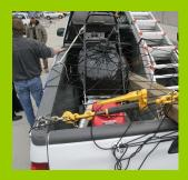
Netting, straps, rope, chain and bungee cords can be used to tie each large item to the vehicle. Since there is nothing in the load that can blow out, a cover is not needed
